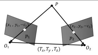
Figure 1. The co-planarity model relating stereo-images.
