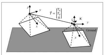
Figure 2. Stereo-images from a UAV platform equipped with a nadir-looking camera while moving at a constant flying height.
