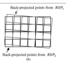
Figure 3. (a) Synthetic grid and simulated 3D object points, and (b) discrepancies between corresponding back-projected points using two ROP sets.
